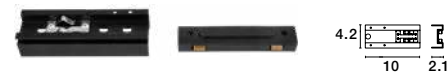
CONNECTOR - 8252015 Mechanical-Electrical Connector Used On Recess & Surface Magnetic Profile To Connect Two Profiles Together L: 10 W: 4.2 H: 2.1 cm
