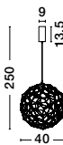
SOLE - 9186905 Titanium Black Copper LED 21 Watt 230 Volt 2403Lm 3000K IP20 Led Chip: 60 Pcs D: 40 H: 250 cm
